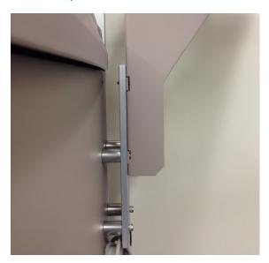
If the handle accessory is present, use both the 1-in. long and 3/8-in. long spacers along with the 2-1/4-in. long screws to provide the necessary clearance.
